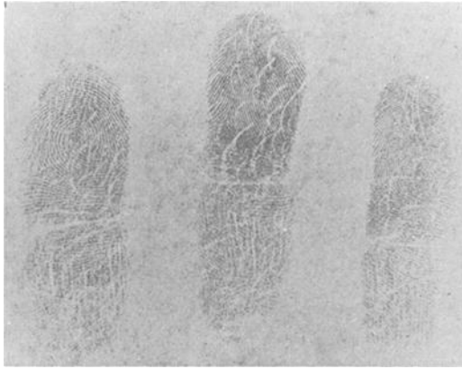
FIG. 4— Photograph of prints after development on Kromekote paper with a fiberglass brush and black fingerprint powder.
