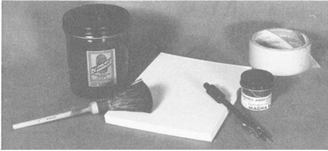
FIG. 2—The materials necessary to lift a print from human skin include a fiberglass brush and black fingerprint powder (left), Kromekote paper (center), and a magnetic brush kit and lifting tape (right).
